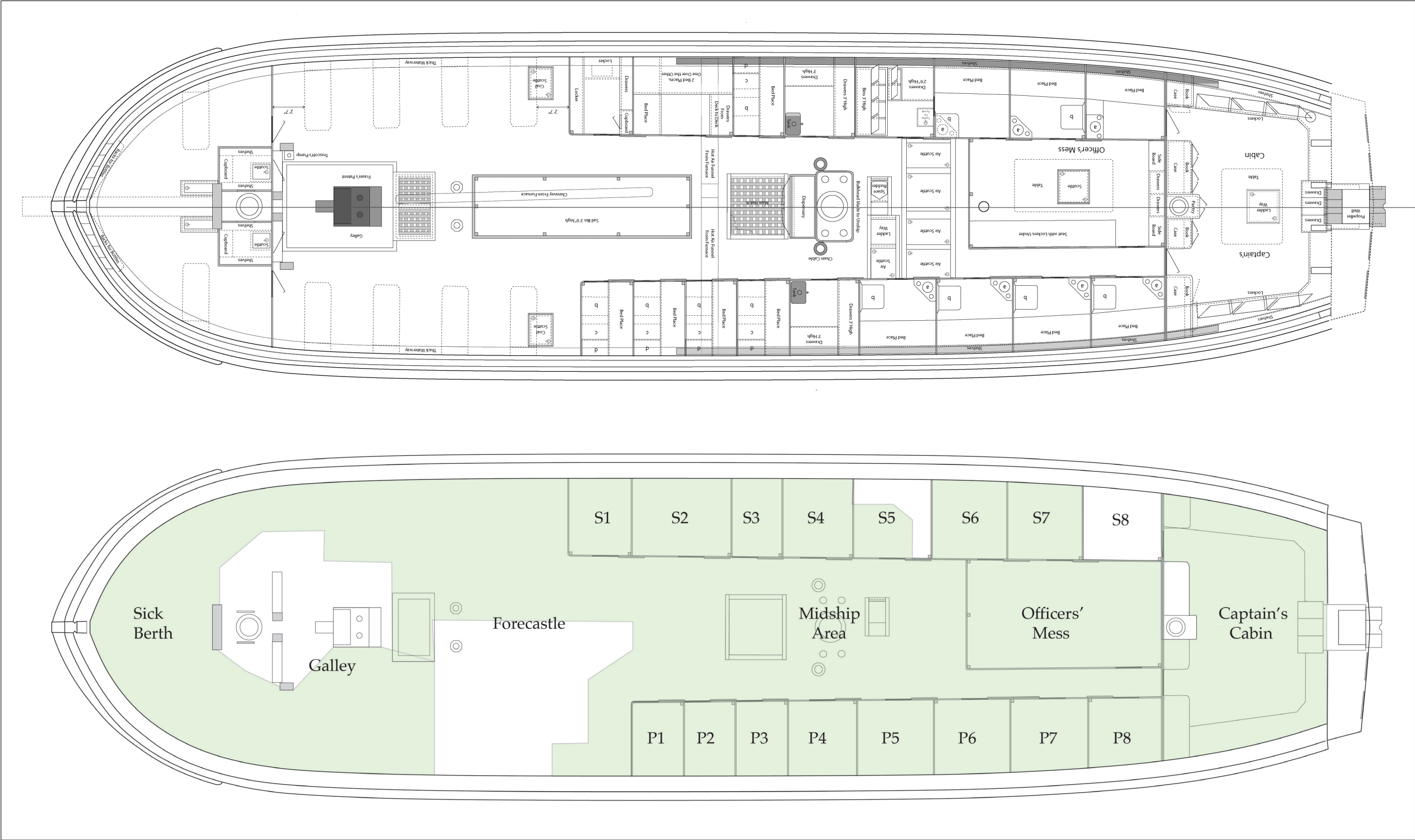
Figure 4.2.4: Top: Terror's lower deck reconstruction by Matthew Betts, based on the Plan of the Terrors Lower Deck , and Profile of the Terror , including modifications from both 1837-1839, and 1845 (Drawing: M. Betts, 2016); Bottom: Key map of Terror's lower deck showing ROV video coverage and naming and coding of discrete spaces. The outline of the vessel is based on Terror's ship plans (NMM, 1837a; 1837b; Betts 2016). Bulkheads and features are drawn based on archaeological data (Drawing: C. Dagneau and R. Harris, Parks Canada).
