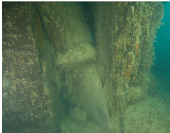
Figure 4.1.2: Terror 's propeller in its working position within the propeller aperture (Photo: M.-A. Bernier, Parks Canada, 90M02819EF).
