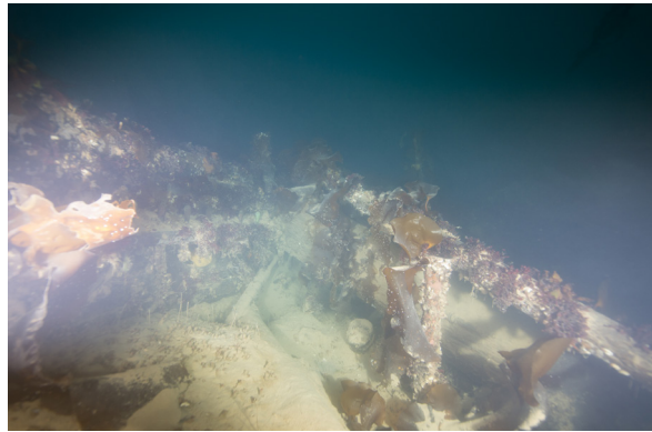
Figure 4.4.2: Terror 's bowsprit heel, stepped in a manner consistent with the Terror 's 1845 modifications (Photo: T. Boyer, Parks Canada; 90M1711EF).
