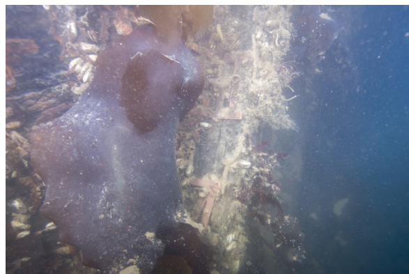
Figure 4.1.3 Rudder post of Terror with copper alloy draft marks "XII" and "XIII" (Photo: T. Boyer, Parks Canada; 90M01494EF).
