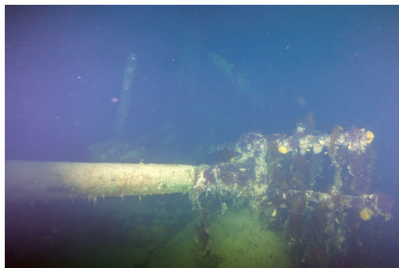
Figure 4.4.5: Possible mizzen topmast with its upper end partly resting on the starboard bulwark (Photo: T. Boyer, Parks Canada; 90M01633EF).
