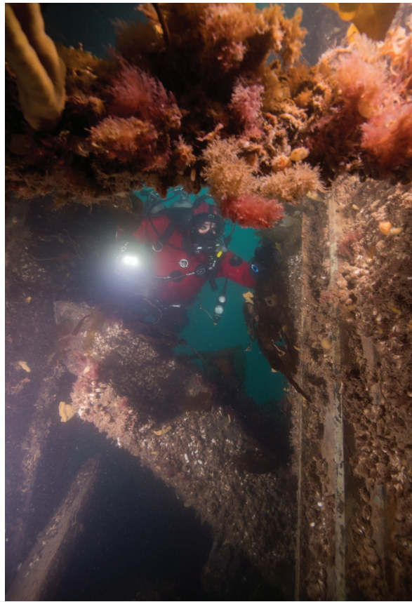
Figure 5.1.2: UAT underwater archaeologist inspects the propeller well of Erebus , including one of the tracks that guided the propeller into position (Photo: T. Boyer, Parks Canada; 89Moo437EF).
