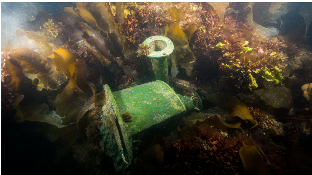
Figure 5.2.5: Partially disarticulated Massey patent bilge pump on the port side of the mainmast atop the wreck (Photo: T. Boyer, Parks Canada; 89M00496EF).
