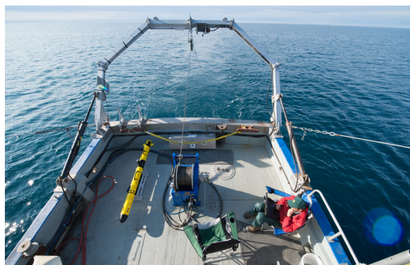
Figure 3.3.1: Towed side-scan sonar operation from the MV Martin Bergmann (Photo: J. Moore, Parks Canada, 51M2684EF).
