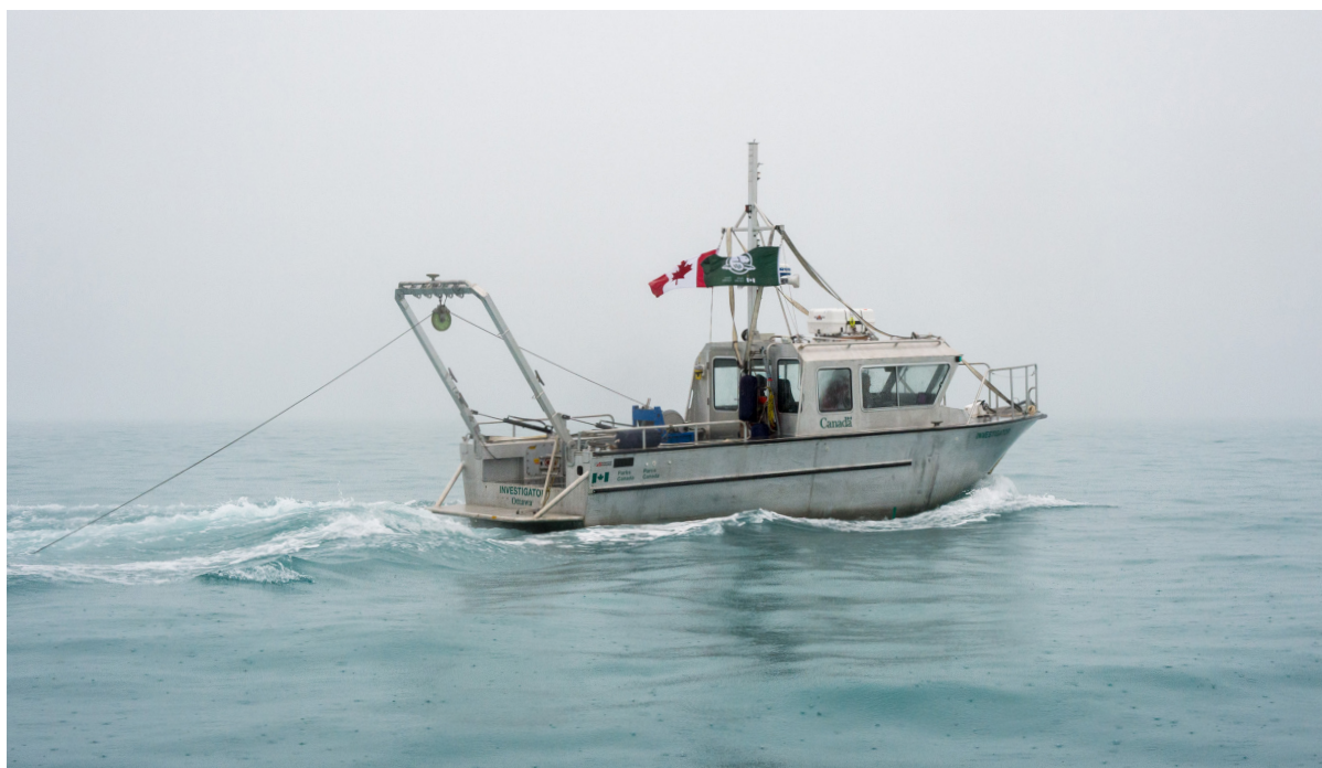
Figure 3.2.2: RV Investigator towing side-scan sonar in 2013 (Photo: T. Boyer, Parks Canada, 51M2495EF).
