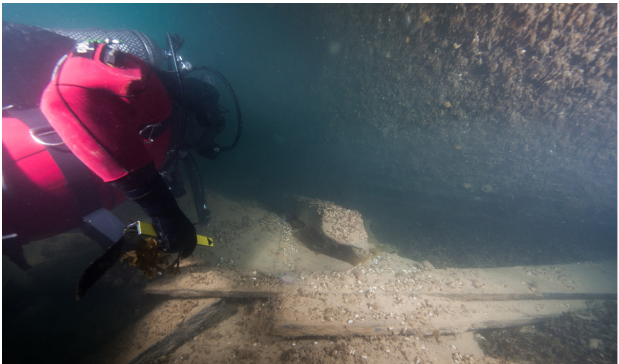
Figure 5.1.1: Scour pocket under the starboard stern quarter of the wreck of Erebus . Mussels growing on the outside hull planking can also be seen (Photo: T. Boyer, Parks Canada; 89M0737EF).
