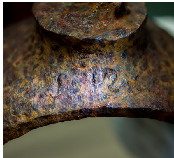
Figure 4.2.2: Close-up of the davit pintle found on shore showing two broad arrow marks and the number 12 (Photo: T. Boyer, Parks Canada; 89MO252EF).
