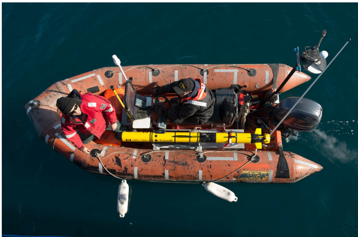
Figure 3.3.4: Ryan Harris (left) prepares to deploy the Iver3 AUV in the southern search area (Photo: J. Moore, Parks Canada, 51M2689EF).
