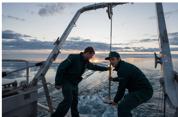
Figure 3.3.3: Retrieval of the side-scan sonar towfish aboard Investigator at the end of a day of survey (Photo: J. Moore, Parks Canada, 51M2848EF).
