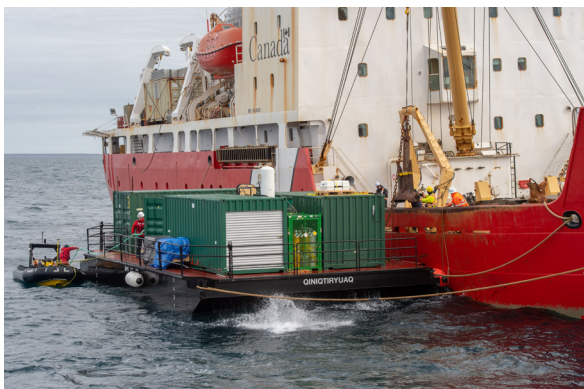
Figure 4.1: The crew of the CCGS Sir Wilfrid Laurier lowers a mooring anchor to the barge Qiniqtiryuaq , while Parks Canada staff set up the mooring lines (Photo: J. Moore, Parks Canada, 89M09435EF).
