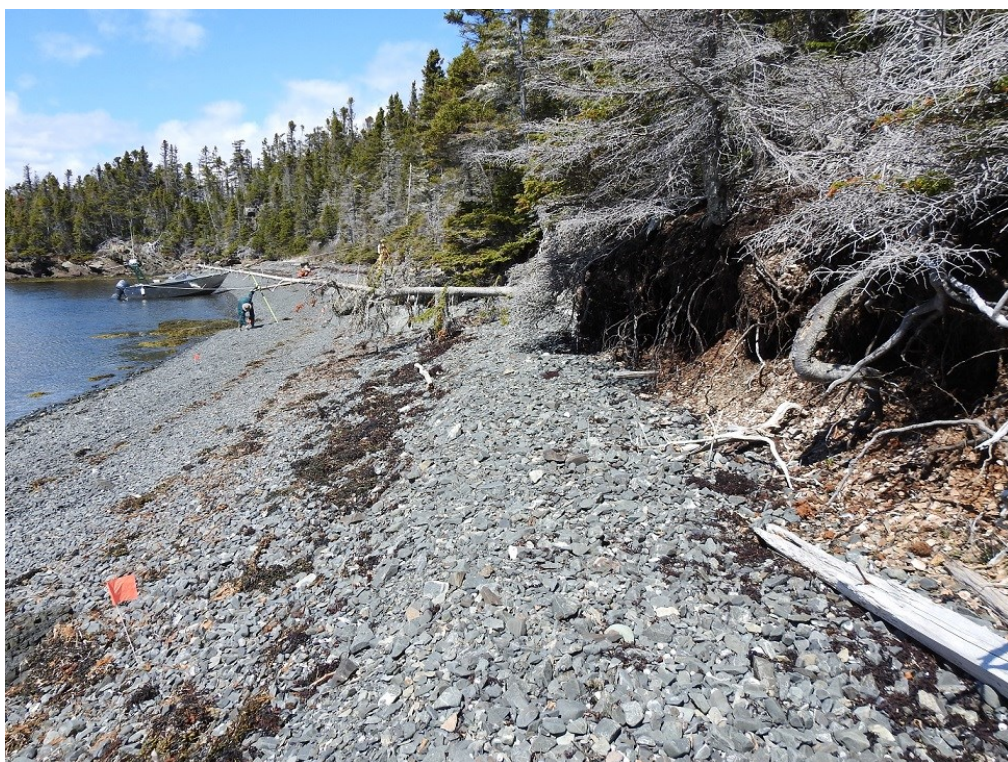
Figure 30: 31A Chandler's Reach: Southern shoreline. Note eroding bank and undercutting of vegetation
