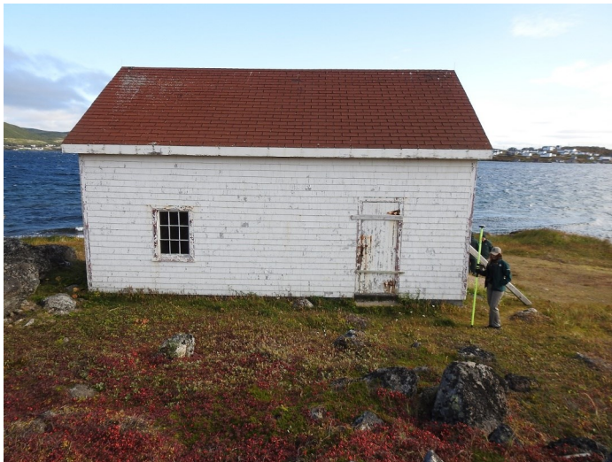
Figure 21: Red Bay NHS (9A12). Surveying assessment area with Juniper Geode GNSS and tablet
