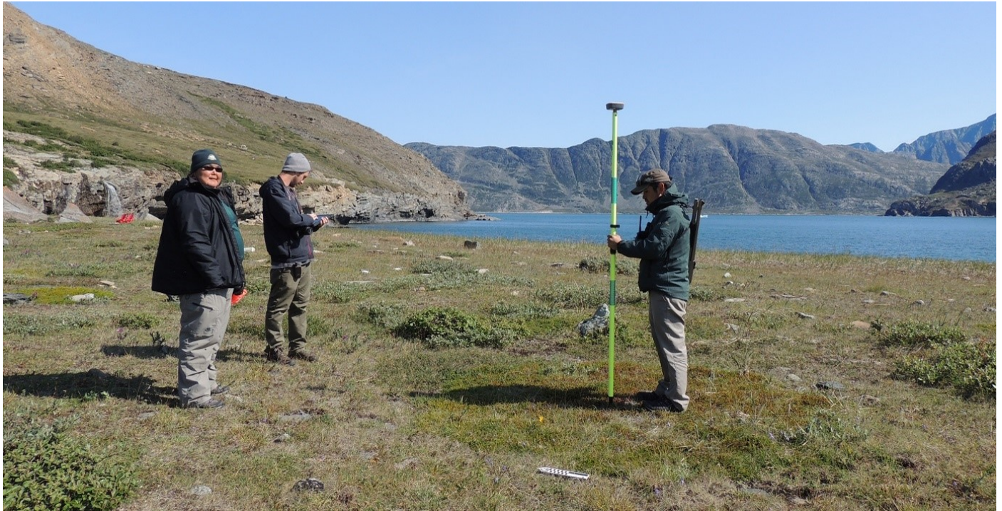
Figure 4: Parks Staff, Nancy Kooktook, Jobie Unatweenuk and author, Wesley Weatherbee recording feature location using GPS/GNSS receiver and Android tablet. Facing east (Parks Canada 2017).
