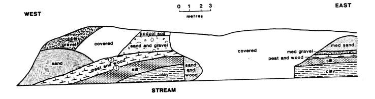
Figure 7. Sketch of stream bank exposure near Nipissing shoreline (SJ-106). Radiocarbon samples indicated by circled numbers.
