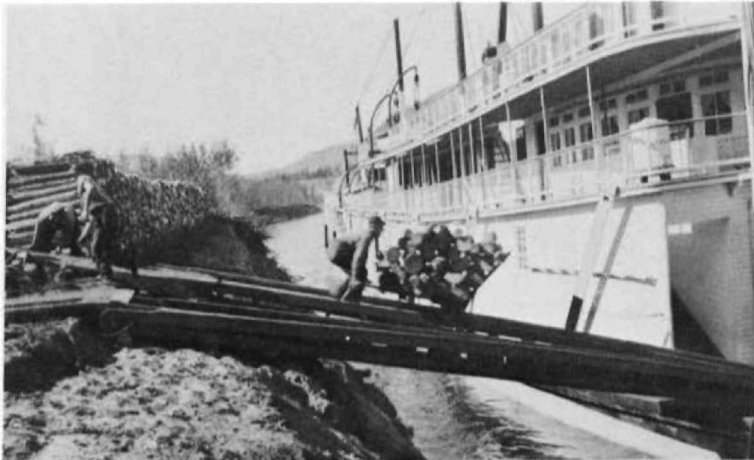
Cordwood being loaded aboard at a riverside wood camp. It was stowed both port and starboard to balance the boat in the water.
