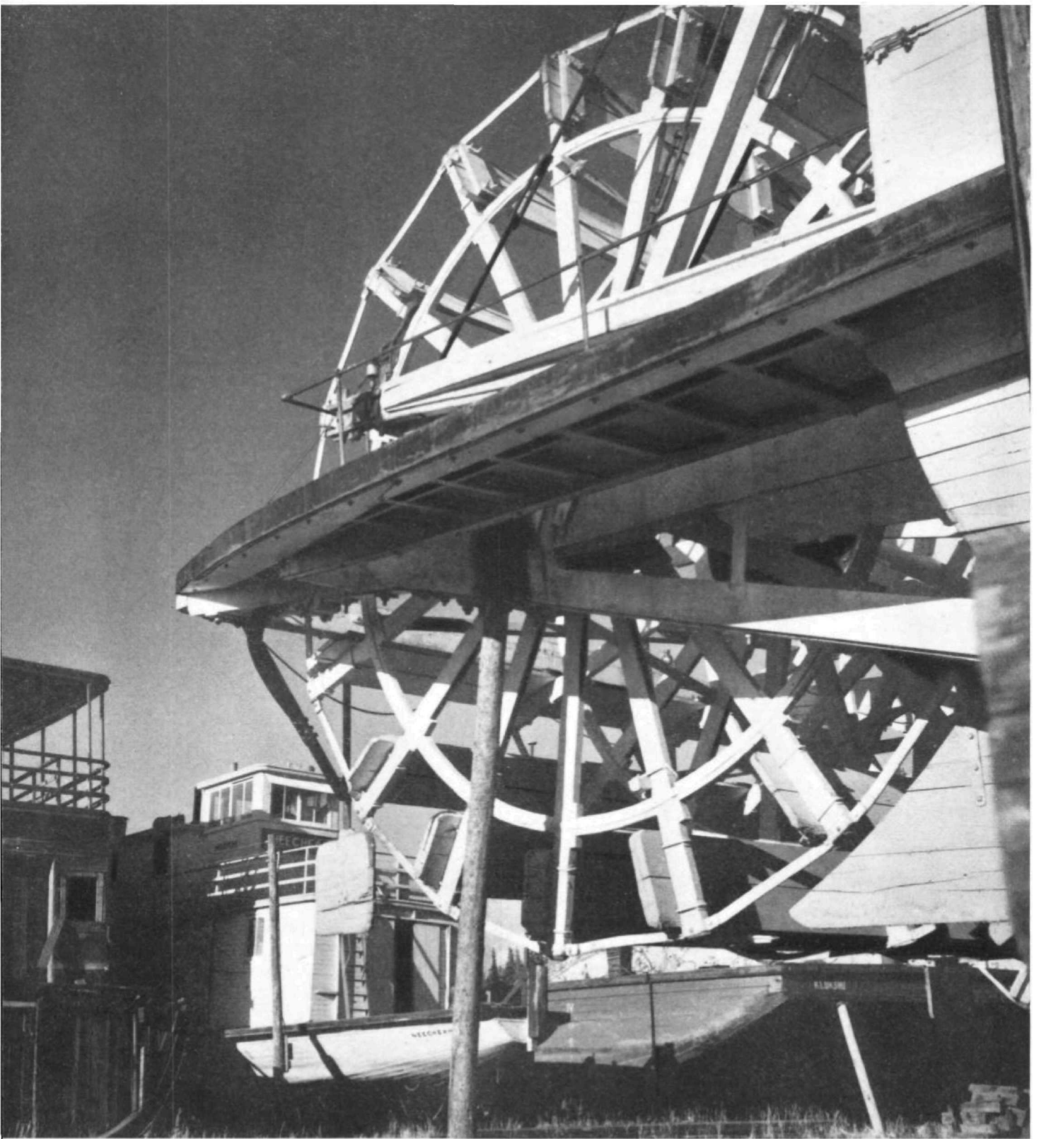
The stern wheel of a Yukon River steamboat in the shipyard at Whitehorse.
