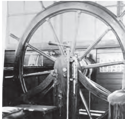
THE “TUTSHI’S” WHEELHOUSE. INSTRUMENTS IN THE WHEELHOUSE INCLUDED A WHEEL AND STEERING LEVER, COMPASS AND A MEANS OF COMMUNICATING WITH THE ENGINE ROOM; SEQUENTIALLY A SYSTEM OF BELLS, A VOICE TUBE, AND A TELEGRAPH SYSTEM. (YA, FRED DUNN FONDS, 83/55, #8)
