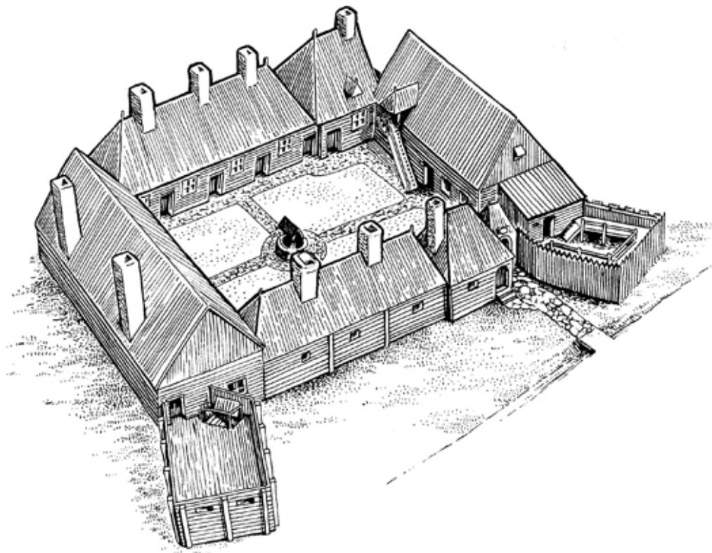
The majority of the Habitation is constructed out of wood. The entire frame and all of the support beams are squared timber joined together with wooden pegs. The roofs and the outside walls are hand-sawn boards. A couple of the roofs have hand-split
