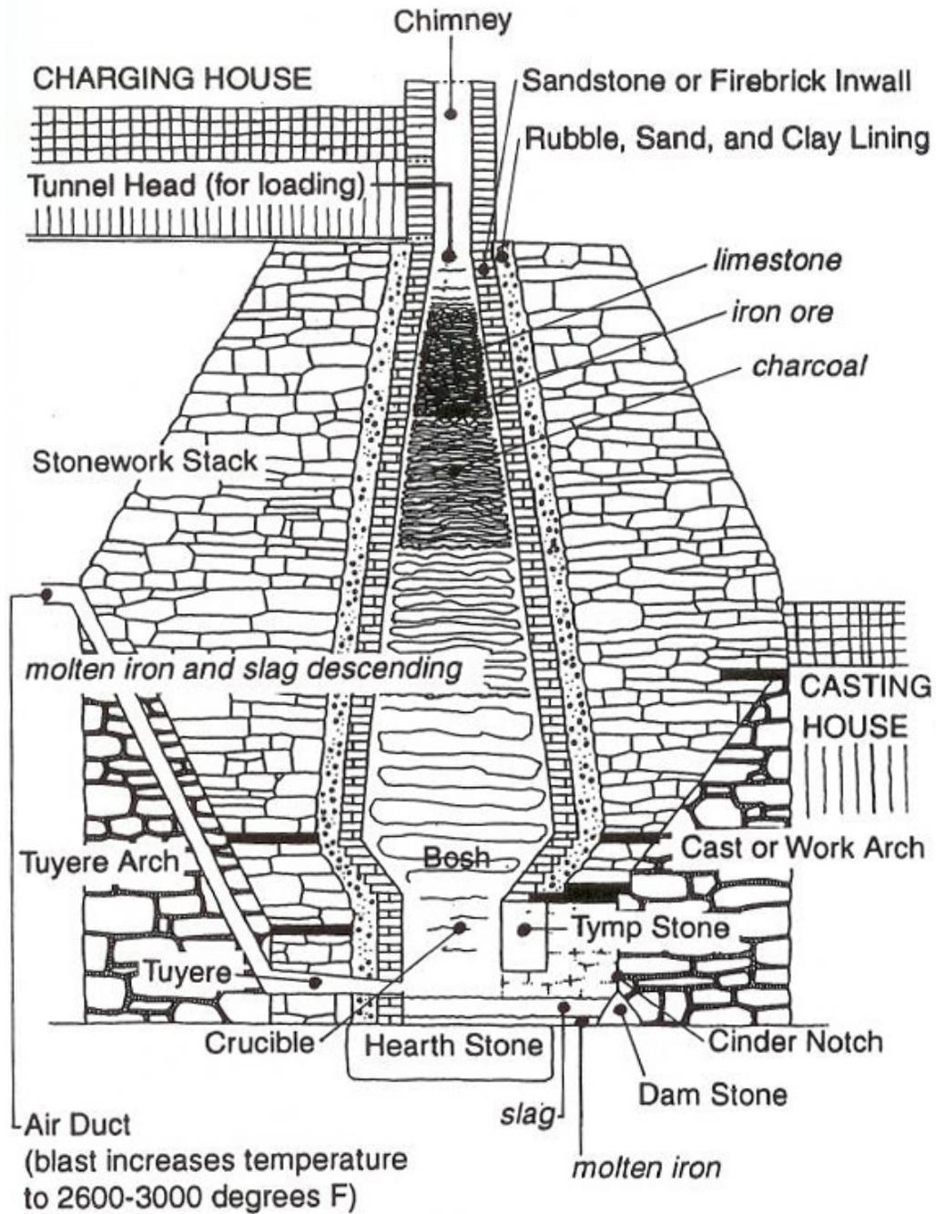
*Fig. 2 Diagram of a cold-blast, charcoal-fueled iron furnace.*
