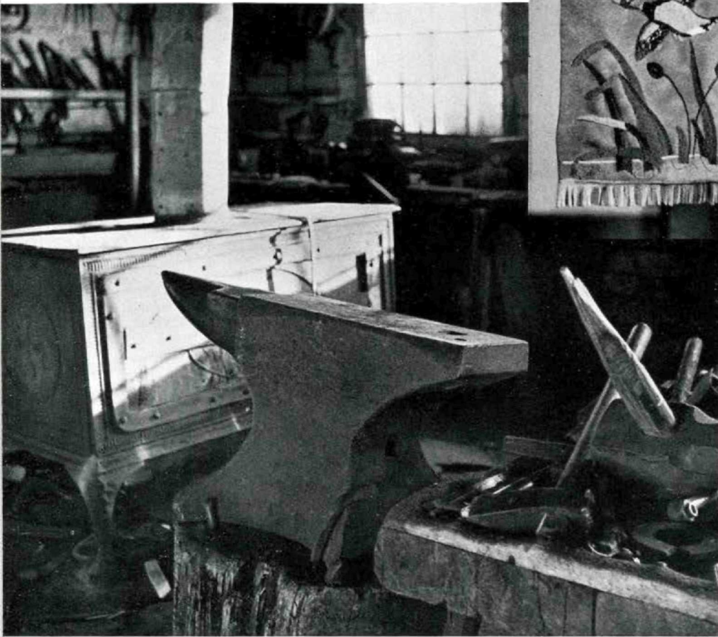
Left: On this old anvil, generations of blacksmiths have pounded out spikes, nails, York boat fittings, door hardware, camp stoves, angle irons, canoe-pole irons, sled hardware, and dozens of other metal articles for use around the post, and on the rivers and trails that lead to it. Behind it is an old Carron stove, used in the fur trade across Canada. R. N. Hourde
