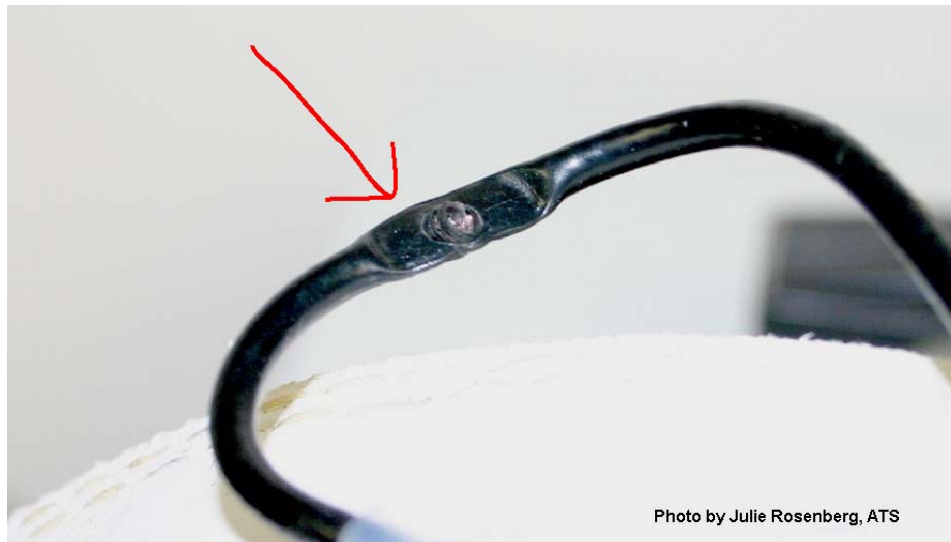
Figure 2. Antenna wire showing damage caused by fastening screw, from collar of study animal F411 (from Obee 2006).
