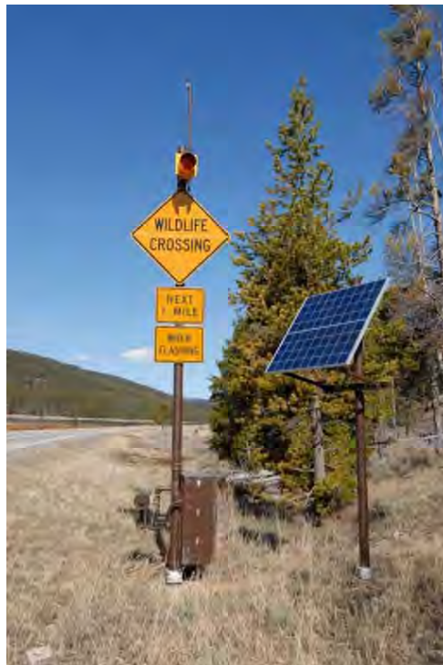
Figure 19: An animal detection system on U.S. Highway 191 in Yellowstone National Park (© Marcel Huijser).
