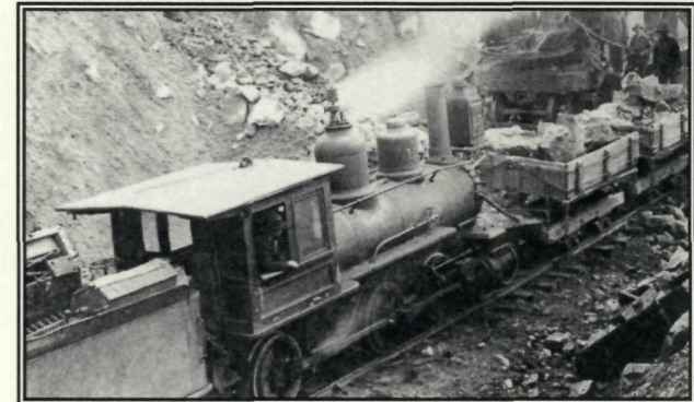
This Baldwin 2-6-0 narrow gauge locomotive worked on the Spiral Tunnels. (Glenbow Archives NA 1285-2)
