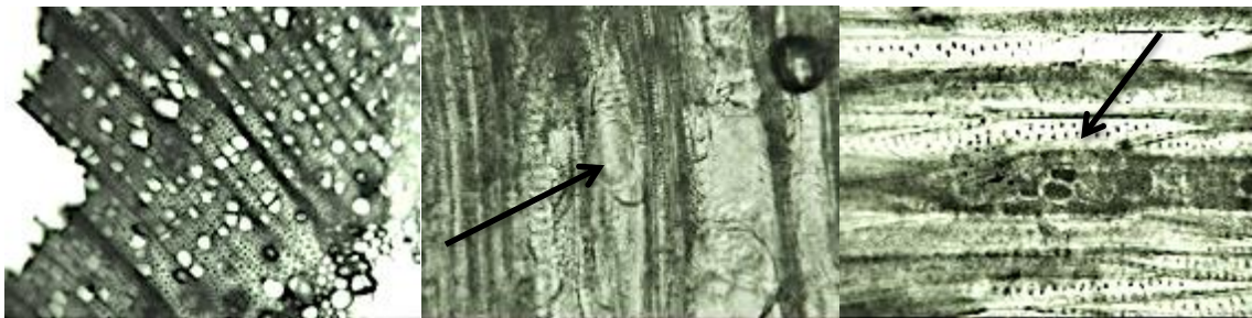
Figure B7. Comparative sample cross section of Sambucus racemosa showing vessel arrangement (left); radial view with simple perforation plate (middle); tangential view of multiseriate ray (right).
