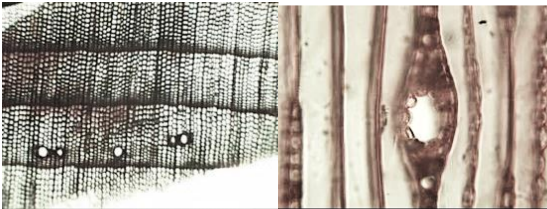
Figure B3. Cross section of comparative Picea sitchensis with longitudinal resin canals (left); Tangential view of fusiform ray 40X (right).
