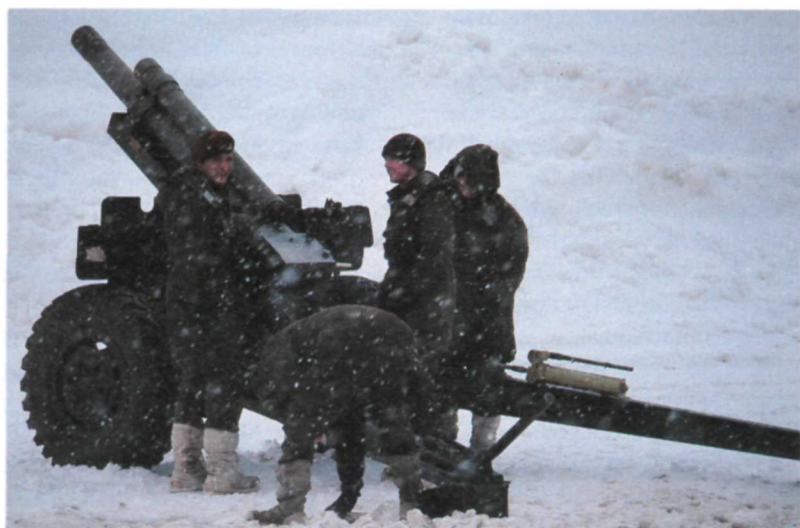
105 mm howitzer used to stabilize avalanche slopes
