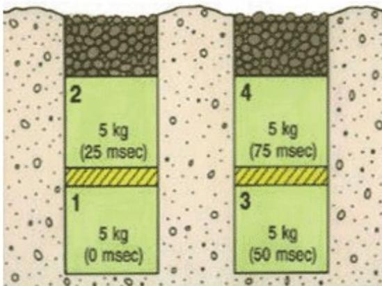
Per Fig. 1: 20 kg total weight of charge; 25 msec delay between charges and blast holes and decking of charges within holes. (Fisheries and Oceans Canada, 2015)
