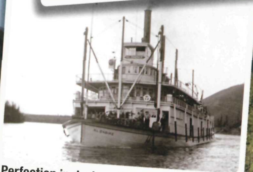
Perfection in design: Although she could carry 270 tonnes of cargo, the S.S. Klondike drew only 1 m (40") – ideal for a shallow, constantly changing river. (Parks Canada / Cy Andrews Collection #42)
