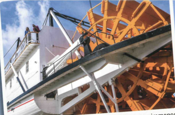
Steam Ship Klondike: Steam generated from an immense boiler powered two compound jet-condensing engines, which in turn cranked the paddle wheel. (Parks Canada / P. Gowdie)
