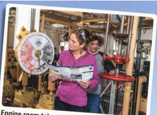
Engine room telegraph: The Chief Engineer received direction from the Pilot in the wheelhouse via telegraph. (Parks Canada / P. Gowdie)
