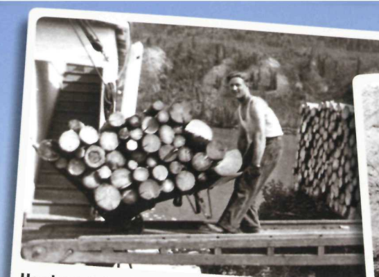
Hard work for deckhands! The S.S. Klondike burned over a cord of wood every hour when steaming upstream. (Parks Canada / G.D. Bissell Collection #232)
